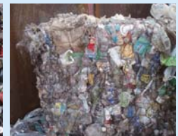
Bad example of pressed steel cans
