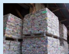
Good example of pressed steel cans
